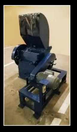
Plastic Waste Management Globe installed its own plastic shredder for processing of clean and dry plastics
